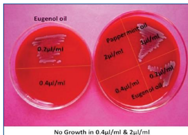
Figure 1. An example of MIC determination, from Thosar et al. [3] .
